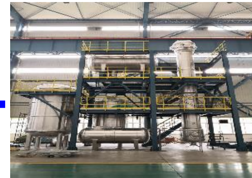
3) Water extraction to remove radioactive impurities
