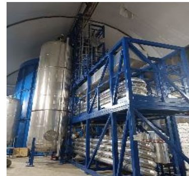
4) Gas stripping to remove Rn and O 2
