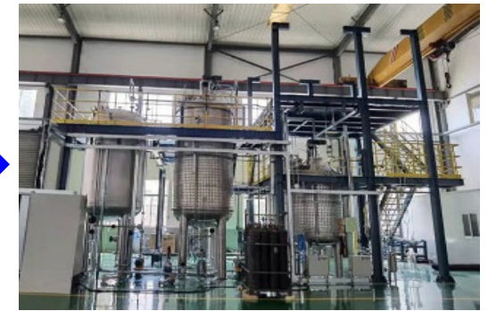
Mixing LAB with PPO and bis-MSB
