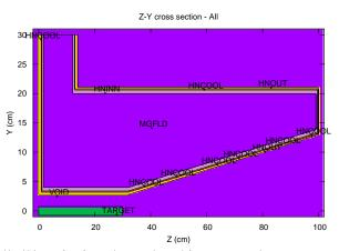
outer skin, thickness: front face  $t_1$ , inner cond.  $t_2$ , exit face  $t_3$ , outer cond.  $t_4$ water channel t5, inner skin t6
