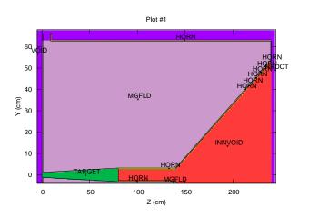
$$\begin{split} E_{\sigma}^{kin} &= 4.5 \text{ GeV} \\ \sigma^{bm} &= 0.4 \text{ cm} \\ L^{lg} &= 80 \text{ cm} \\ R_1^{lg} &= 1.2 \text{ cm} \\ R_2^{lg} &= 3.2 \text{ cm} \\ z^{lg} &= 0 \text{ cm} \\ L_2^{hn} &= 60 \text{ cm}, \\ L_2^{hn} &= 100 \text{ cm}, \\ R_2^{hn} &= 50 \text{ cm}, \\ R_2^{hn} &= 50 \text{ cm}, \\ t_1 &= 1.0 \text{ cm}, \\ t_2 &= 300 \text{ kA} \end{split}$$
