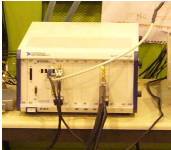
IPHC-NI DAQ : 1 x Flex RIO board in PXI Express crate
