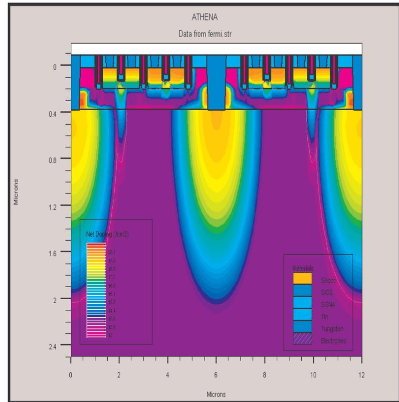
Diode simulation in Flexfet process
