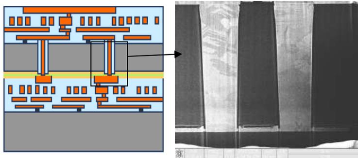
IMEC, Pitch  $\sim 10\mu\text{m}$ , with glue
