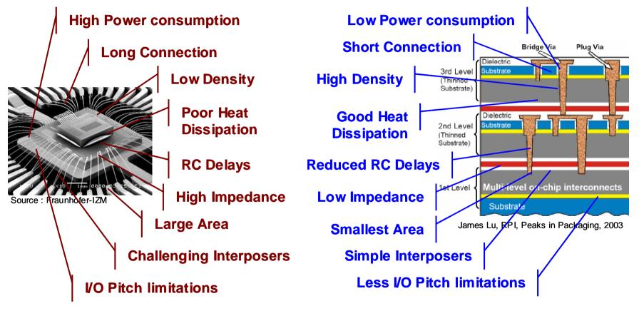
TSV interconnects provide solutions to many limitations of current SiP and Chip Stacking methods.
