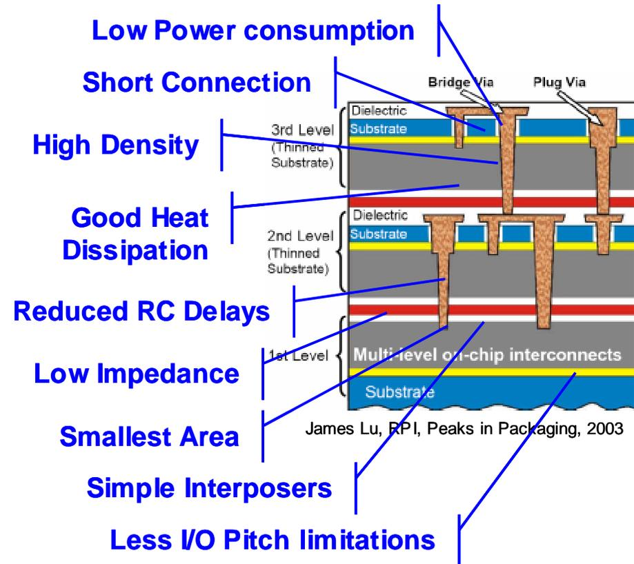
TSV interconnects provide solutions to many limitations of current SiP and Chip Stacking methods.
