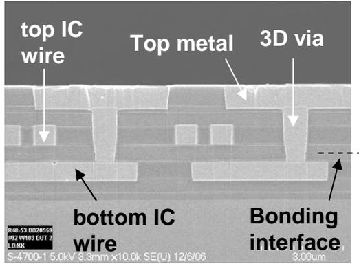
**CEA Léti - MINATEC / Alliance, SiO<sub>2</sub> bonding, pitch ~5µm (SOI)**
