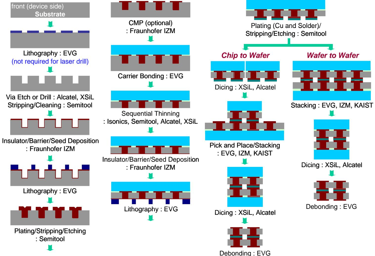
We are considering both via-first and via-last approaches (start with via-first approach). This process flow is not for licensing, but is an example of process and equipment flow for demonstrating chip integration with consortium members' technologies.
