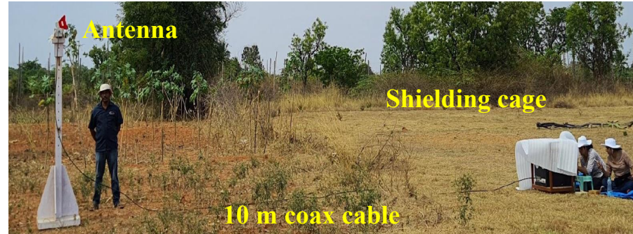
Shielding cage to enclose the Laptop, Spectrum analyzer and the receiver
