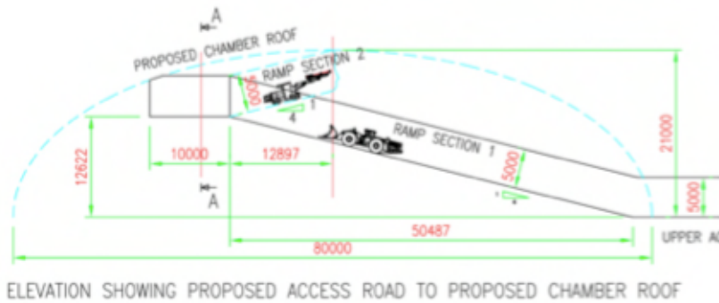
Fig. G4.3.3 First stage construction methodology for formation of the dome roof.
