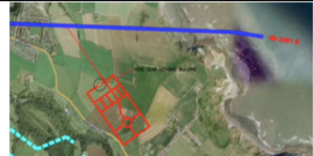
Fig. L6.4.1 shows the expected position and layout for the LENA cavern
