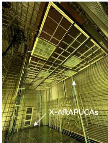
PDS installation in ProtoDUNE-VD
