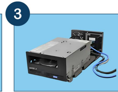
3 Attach a benchtop power supply and serial cable to the back of the drive
