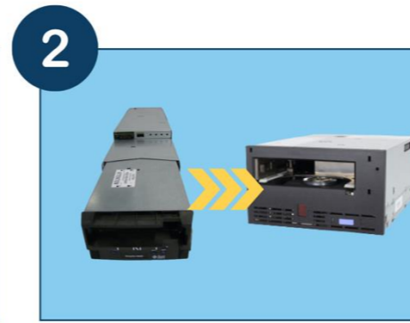
2 Remove the LTO drive brick from its original drive sled assembly
