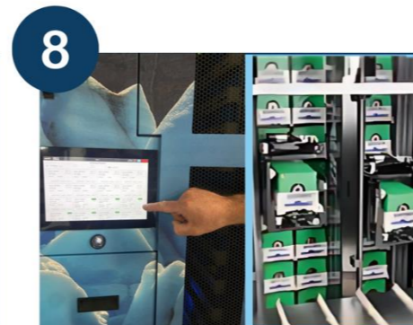
8 One last final onboard test is completed in the Spectra Cube using the robotics and onboard drive test utility
