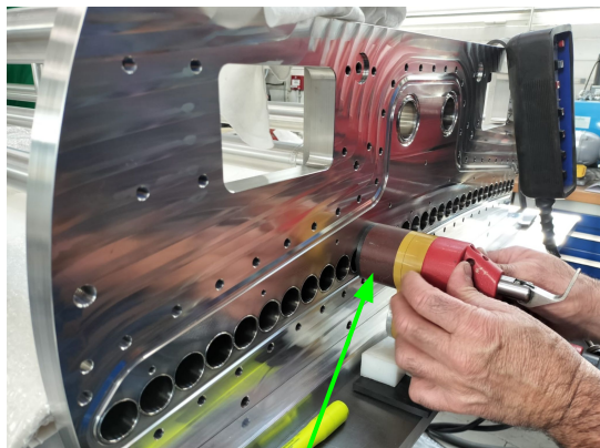
Automatic welder (power and rotating speed pretuned)
