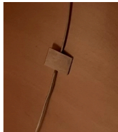
^{210}\text{Po} source (5.3 MeV alphas) located behind 2 mm diameter hole in the cathode
