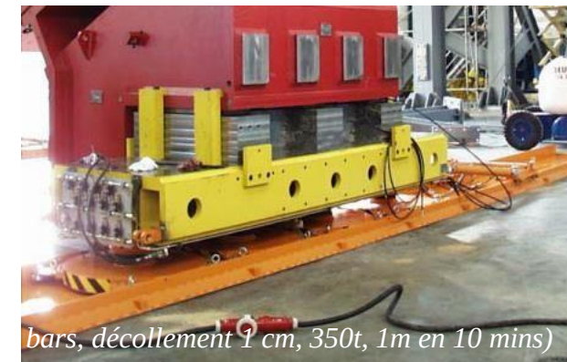
Air-pad, rail de guidage, vérin hydraulique
