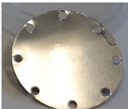
TaN 2.8 \cdot 10^{18} atoms/cm 2 deposited on 7.8 \cdot 10^{17} atoms/cm 2 of high purity Ta interlayer Tantalum substrate
