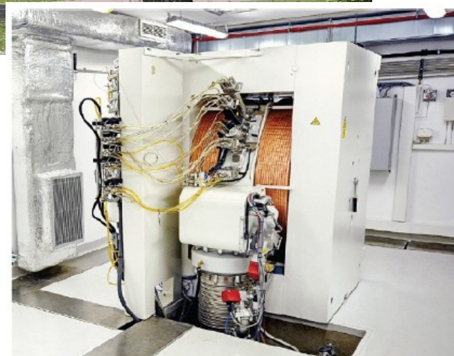
GE PETtrace p/d medical cyclotron Providing protons or deuterons (16.5 MeV/ 8 MeV)
