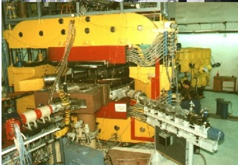
U-200P heavy ion isochronous cyclotron, accelerating ions up to mass 40 (B to Ar) to the energies \sim 10 MeV/A and Alpha internal beam, 32 MeV
