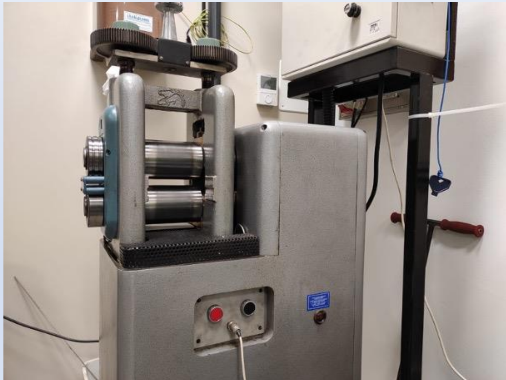
Cold rolling mill
