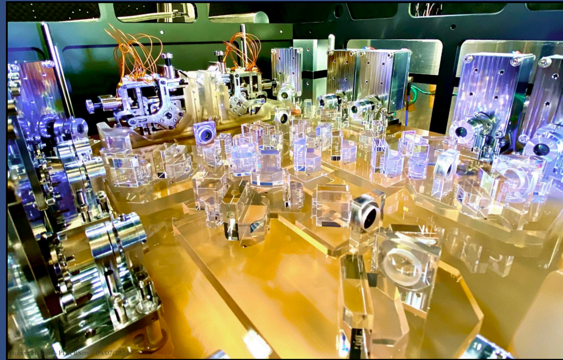
ZIFO example: zerodur slab with optical contacted components
