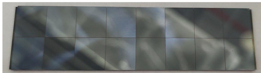
Bump Bonding Process Verification with Dummy Dies
