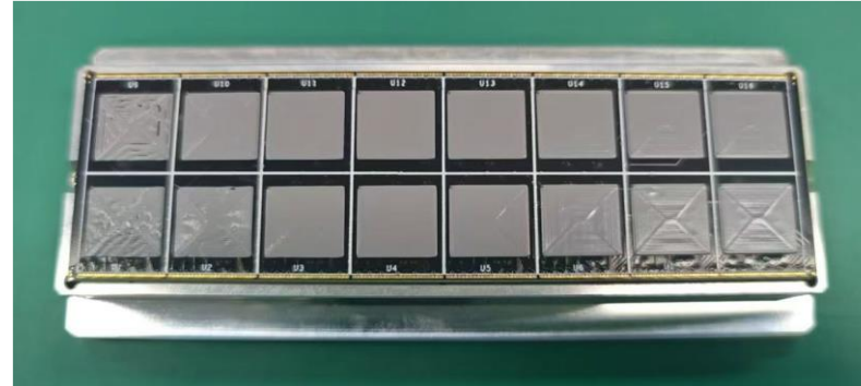
Dispense Glue on the Wire-Bonding Board
