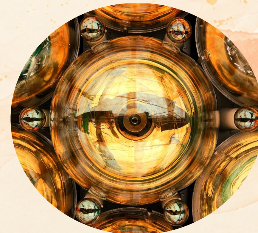
LPMT surrounded by SPMTs
