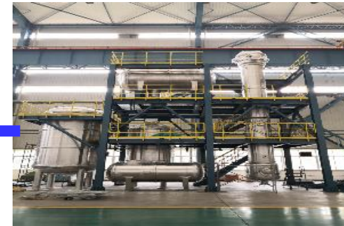
3) Water extraction to remove radioactive impurities
