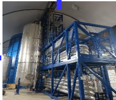
4) Gas stripping to remove Rn and O 2
