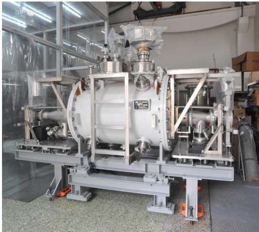
In-house-made 500 MHz cavity and module made in 2011, stable operation since 2017
