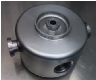
325 MHz Spoke cavity (beta 0.21)
