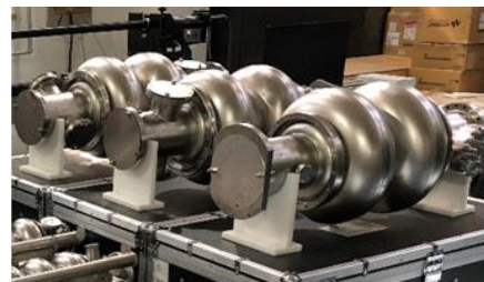
650 MHz test cryomodule with 2x2-cell cavities. Beam test soon.
