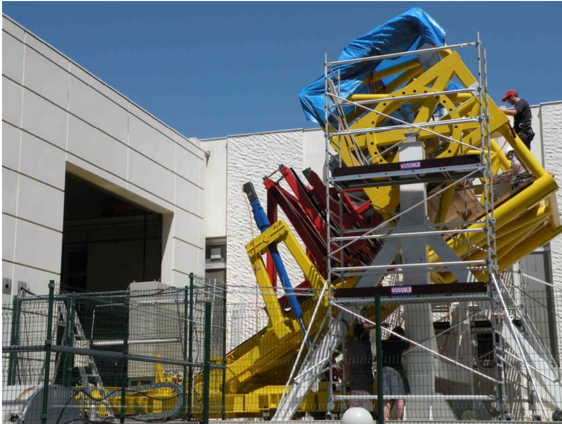
Test of unloading in the lab with the dummy camera and a dummy end of the telescope.
