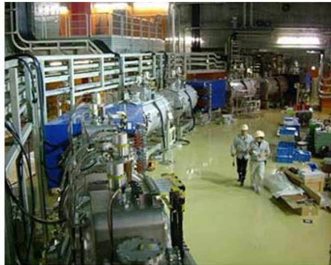
Figure 4: Photographs of the first stage (left) and second stage (right) of the BigRIPS separator
