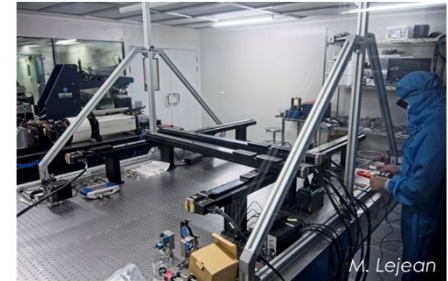
Figure 1: Birefringence bench setup ongoing
