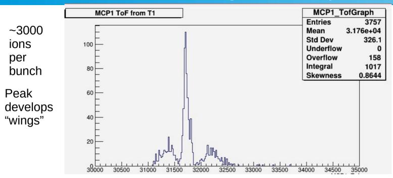
Three peak structure at 200 rev with high beam intensity (Na + Mg)
