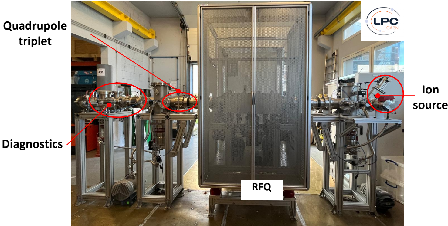
RFQ1P test bench at LPC Caen (w/o the HV cage)
