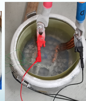
HTS ribbon in different configuration under resistivity test in Ni bath (77 K)
