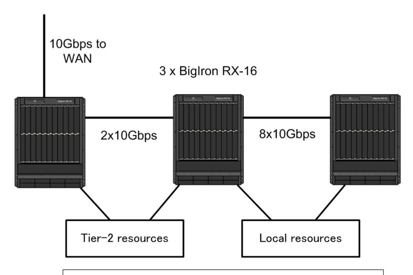
8 x 10Gbps is the limit of link aggregation for this switch
