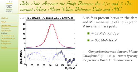
This shift is corrected by multiplying the curvature of the track by a *momentum scale factor*.
