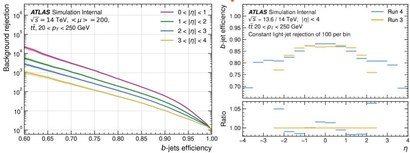
Left: ROC curves for Run 4 tagger in multiple  $|\eta|$  slices. Right: b-efficiency for Run 4 and Run 3 taggers as functions of  $\eta$ .
