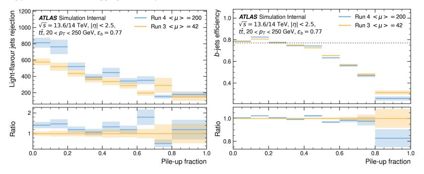
Both Run 3 and HL-LHC b-jet efficiency strongly impacted by PU fraction. Overall **similar response to PU** between the two taggers.
