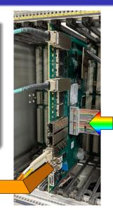
Timestamp **clock** and **reset** signals are sampled by ReBo and written in data flow
