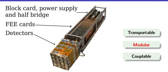
**16 telescopes**, together with **front-end electronics**, form a **block** operating in **vacuum**.
