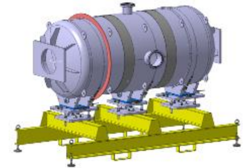
Mock-up Ø850mm to validate assembly strategy
