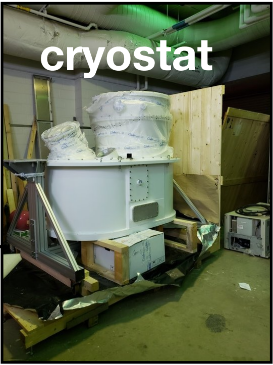
Modified US Cryostat adapted for filled arrays LEKID optics. Lead: Néel
