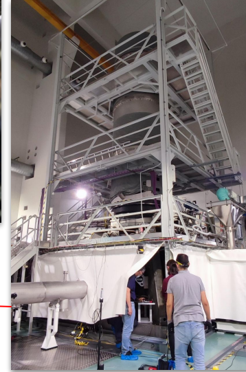
Virgo “end tower” and 42 kg suspended mirror
