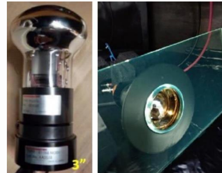
mPMT module: 19 single PMTs of 8cm
