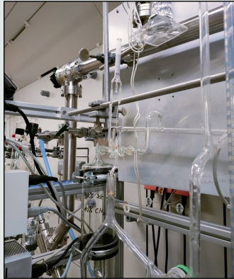
Testing gas isotope composition with a proportional counter
