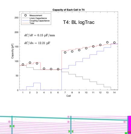
$L_i$  is the length of the i-th trace from the connector, bringing the **Self-Capacitance**.
