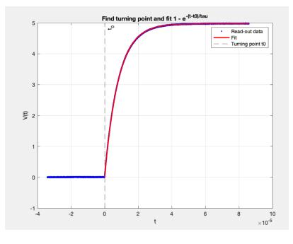
• RC Series Circuit voltage:  $V_c(t) = V(1 - e^{-t/\tau})$
