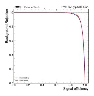
FusionNet performs as well as particlenet in p-p but uses only charged particle information
