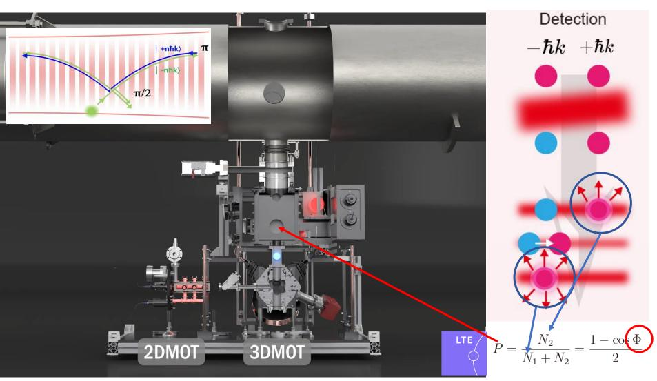
1 loop =1.1s 300ms loading time; 800ms free flight; 4.8E7 atoms in 3DMOT@loading; 1E6 atoms/s flux@detection
