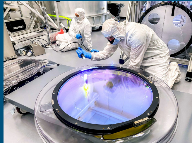
One of the 6 huge filters for the Rubin Observatory LSST Camera being inspected at SLAC National Accelerator Laboratory.
