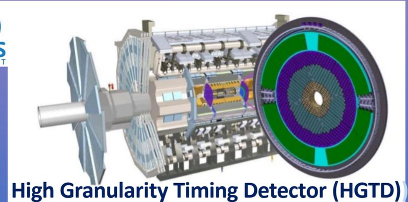
**High Granularity Timing Detector (HGTD)**
