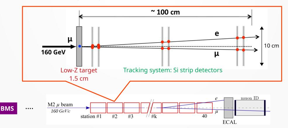
After CERN Long Shutdown 3 (2027-29): full apparatus with 40 stations
