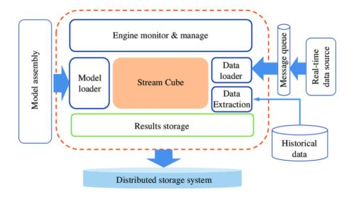
The ePIC detector's streaming architecture opens new possibilities for fast analysis, but demands a shift in how we process data. We're moving from post-processing to real-time processing, integrating AI and calibration algorithms on-the-fly.
