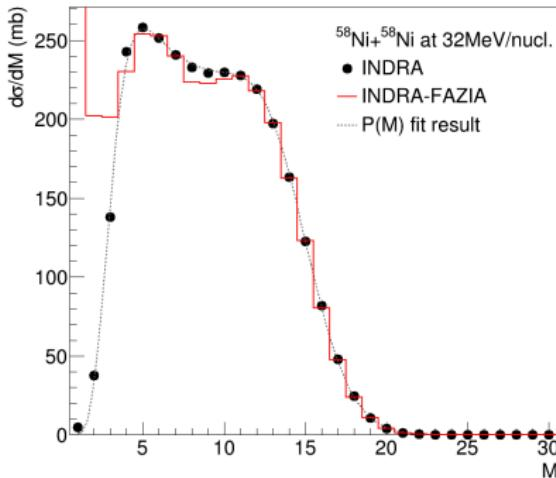
Fit result on multiplicity  $M$  of identified and unidentified particles in INDRA rings 6-17 for  $^{58}\text{Ni} + ^{58}\text{Ni}$  at 32 MeV/nucleon on INDRA dataset
