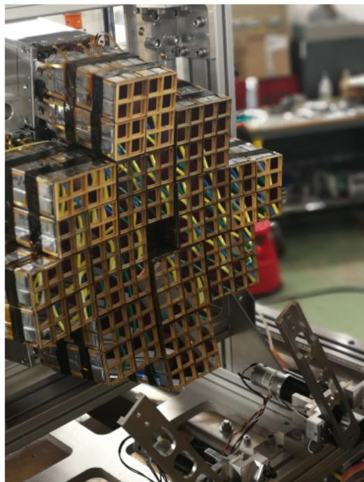
**FAZIA** (*Forward-angle A and Z Identification Array*): optimal ion identification in the Fermi energy domain.
