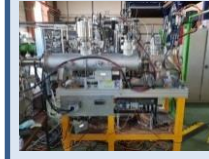
ARIBE: characterization of Ar 8+ beam at 30 keV and commissioning of beam focusing prototype
