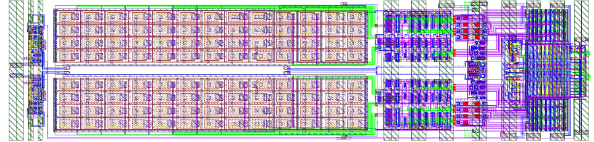
Figure 5. Layout of a single channel of 10-bit SAR ADC.
