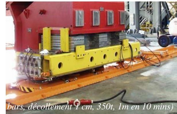
Air-pad, rail de guidage, vérin hydraulique
