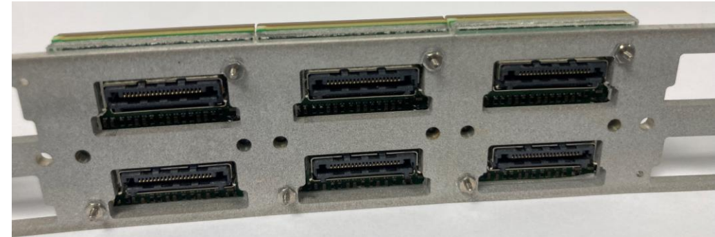
Three CC-EC fixed to the aluminum prototype of the mechanics of the focal plane
