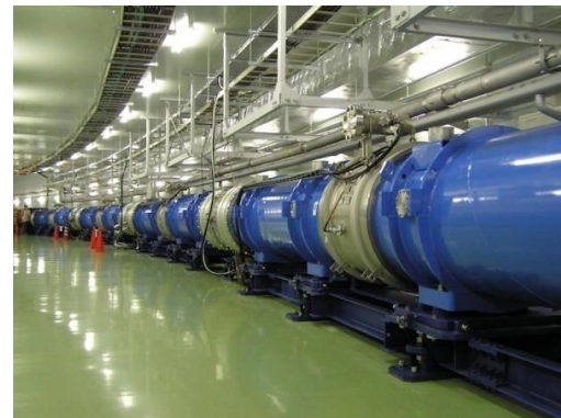
particle accelerator to create neutrino beam
