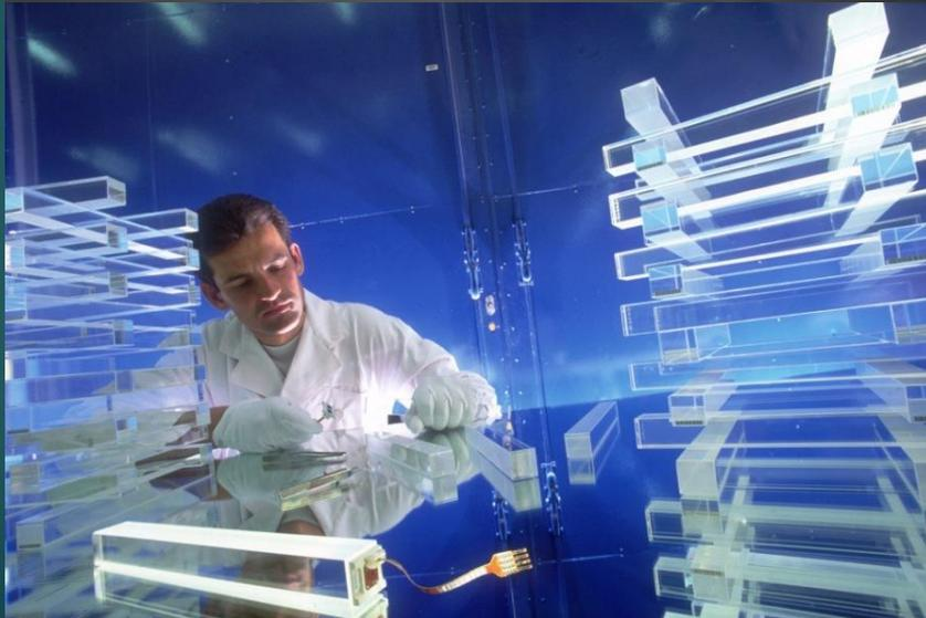
The high energy resolution electromagnetic calorimeter (ECAL) measures the energy of photons and electrons. It is composed of  $\text{PbWO}_4$  (lead tungstate) crystals.
