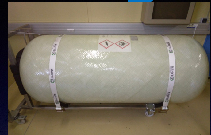
Mahytec tank (for H 2 storage) (L=1.8 m, D= 0.84 m, V=0.85 m 3 , P≤60 bar, 10 k€)
