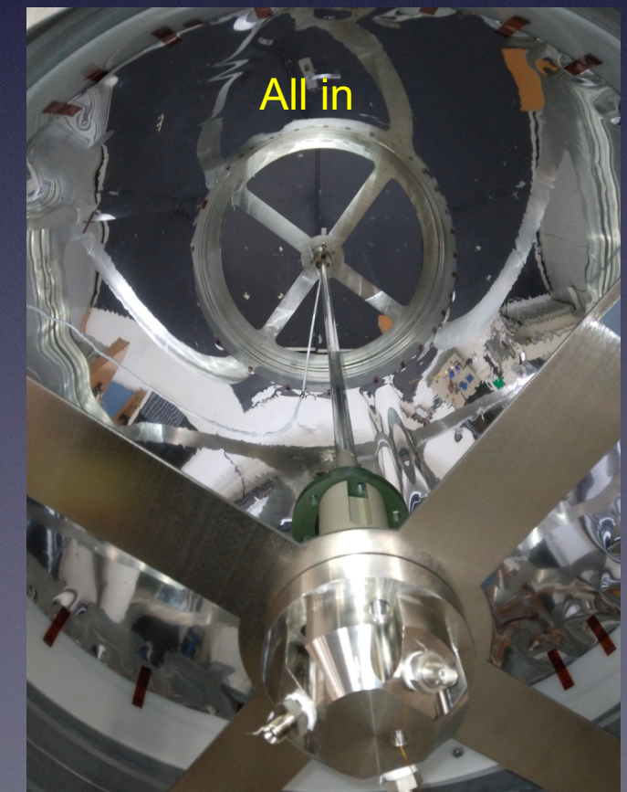
Mahytec tank (for H 2 storage) (L=1.8 m, D= 0.84 m, V=0.85 m 3 , P≤60 bar, 10 k€)
